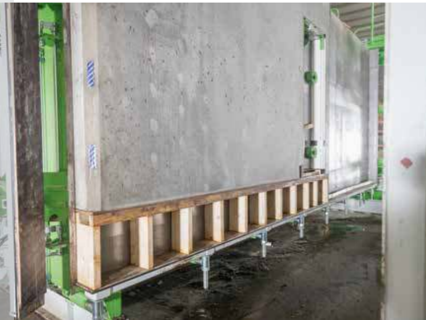
Casting to desired size with smart side forms
